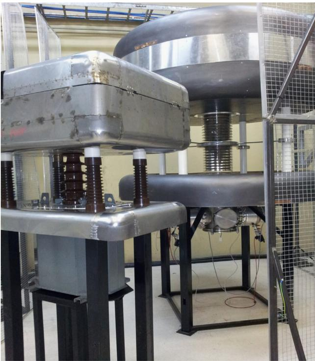
**Fig. 2.** Assembled and high-voltage tested 200 kV accelerator.
