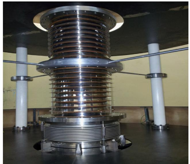
**Fig. 3.** Accelerating column composed mainly of two high-voltage and vacuum tested tubes.
