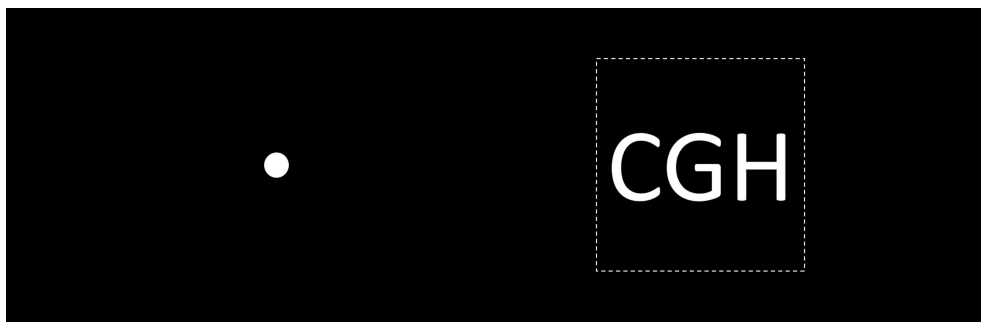
Fig. 2. Schematic of the mask composed by a pinhole and a computer generated hologram. To improve visualization the pinhole has been enlarged from its actual size. By blocking the pinhole we obtain the reconstruction of the hologram and unblocking we obtain the interference pattern of the light diffracted by the pinhole and the reconstruction of the hologram.
